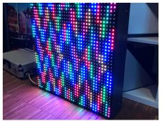
One square metre of the P16 LED film has a power consumption of only 180 watts in video mode.
