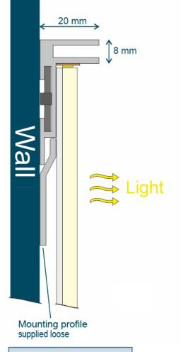
Available with printed and ready-made tensioning fabric on request. Particularly flat LED tensioned fabric frame for backlighting textile prints for indoor use.
