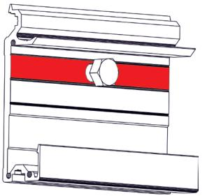
Stay within the screw field marked in red. Any number of fastening points can be set here.
