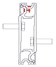
Secure against possible lateral displacement with 4.8 x 19 mm self-tapping screws.
