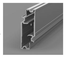
The geometry of the profile not only allows the advertising system to be latched to the wall in a wind-proof manner, but also ensures a very high load-bearing capacity at the same time. We will be happy to provide our tensile test for the purpose of project statics upon request. Due to the low wall thickness of 35 mm, a drainage behind the advertising system is guaranteed. Subsequent height adjustment of the advertising system by up to 10 mm is possible.
