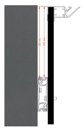
Attach mounting profile to the wall approx. 2 mm deeper than mounting profile on the frame.
